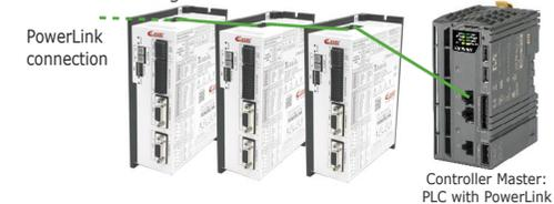
Drives control through command by master controller.
