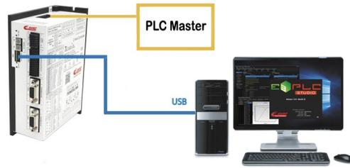
Ever co. proprietary PC Software Tools for easy and quick configuration or programming, real time debug and supervision of each system
