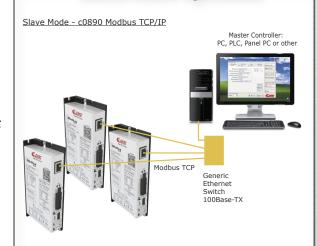
Drive control through commands by Master Controller. Suitable for multi axes systems (up to 127 drives). Built in powerfull Motion Module functionality assures perfect synchronization among axes and reduces Master Controller workload
