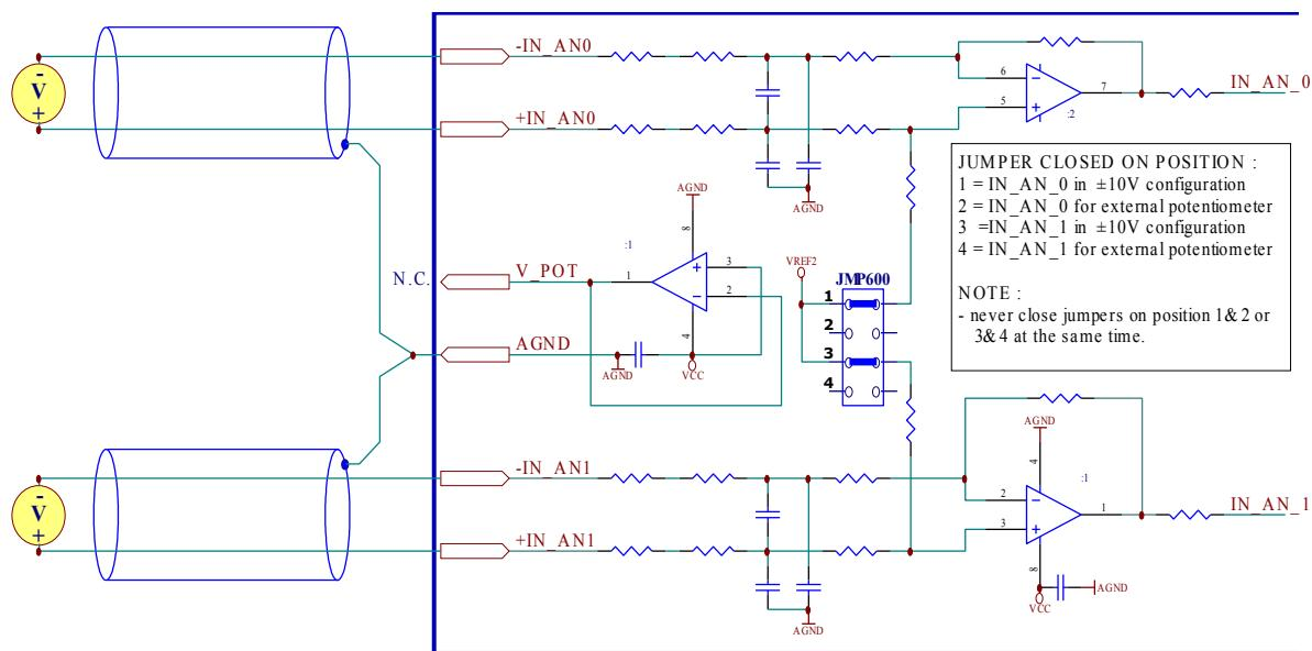
Analog input for potentiometer connection.
