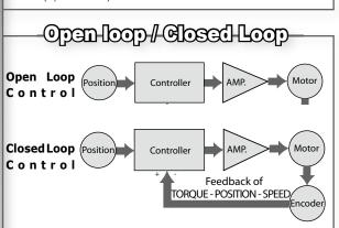
Better control compared to both an open loop stepper solution and a servo-controlled brushless solution
