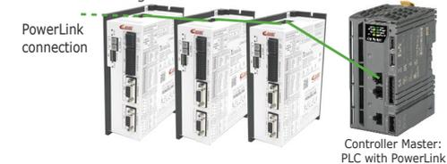
Drives control through command by master controller.
